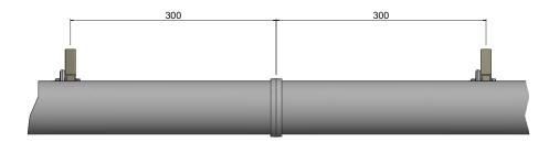
Preparation:- For Best Results Fix Brackets within 300mm Either Side of Join
