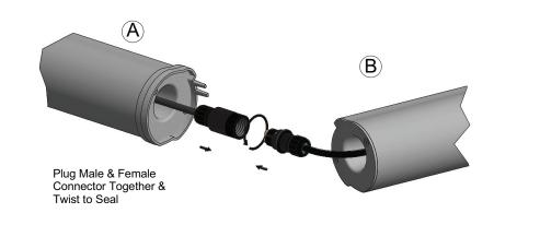
Feed Cable Into IP 67 Grommet
